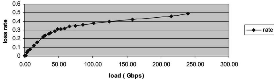
Graph 2. Loss rate as function of load.
