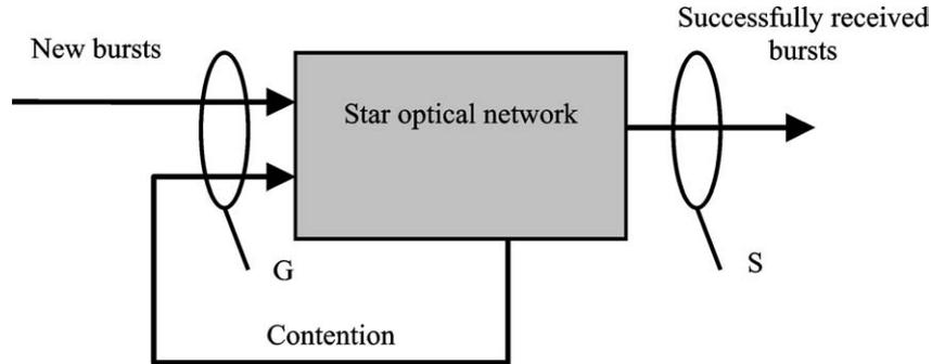
Figure 2. A star optical network with retransmission scheme.
