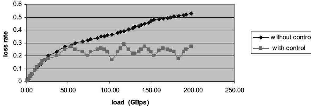
Graph 3. Loss rate as function of load with and without congestion control.
